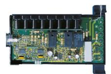
All Weishaupt W series burners are fitted with digital combustion managers as standard, whose microprocessors control and monitor all burner functions. The result: Weishaupt burners are easy to use, precise and safe.
