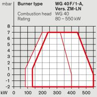
Capacity graphs in accordance with EN 676. The ratings are based on an installation altitude of 0 m. An altitudebased reduction in capacity of approx. 1 % per 100 m above sea level should be taken into consideration.
